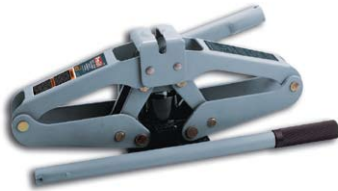
T-9400 2,200 lbs. rated capacity Hydraulic Scissor Jack Hydraulic Mechanism (with carrying case) Lifting Range: 4-3/4" - 15"
