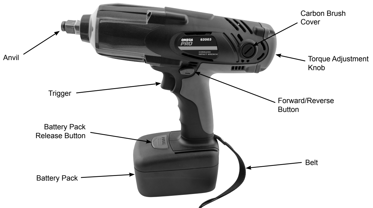
Fig 1. 82003 Impact Wrench components.
